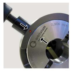
**Note** The clamp shell has been installed correctly, if it is locked in place. If the clamping shell is not locked, this fact can be rectified by a gentle turn of the clamping shell.
