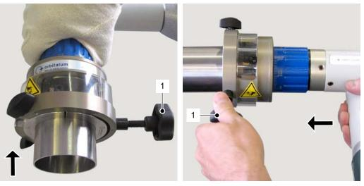
Clamp tube with RPG Electric: tube to machine
