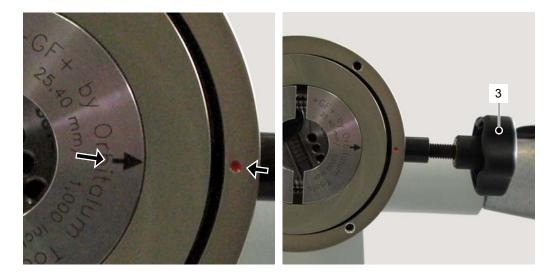
**Note** The clamping shell has been correctly installed, if it is locked in place. If the clamp shell is not locked, this can be rectified by a gentle turn of the clamp shell.
